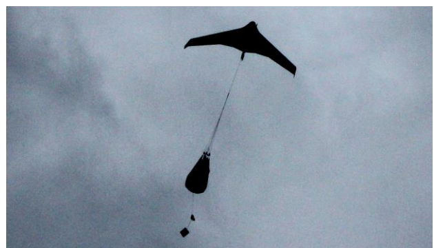
Figure 4: The C-Astral Bramor UAV during the initial deployment of its landing parachute.
