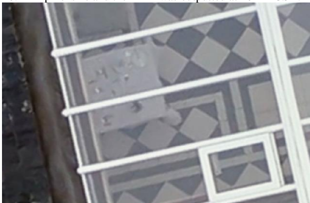
Figure 6: The detail of 1cm orthophotography can be seen here. This is a view looking down through the atrium over the dining area of the surveyed hotel. Note the cutlery on the table.
