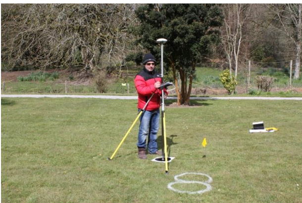
Figure 2: The stabilised Trimble GoeXR Network RTK GPS used to get the coordinates of the target centres.
